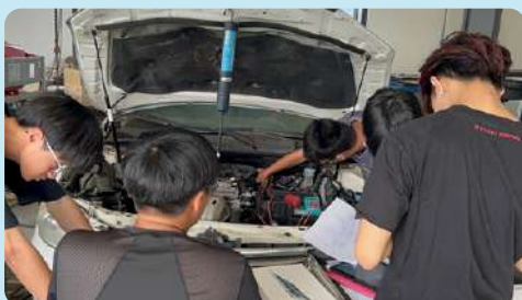
Practical Vehicle Diagnostics and Repair: Students used automotive diagnostic instruments, multimeters, automotive oscilloscopes, and other equipment to inspect real vehicles, identify malfunctions, and carry out troubleshooting. Through this practice, they acquired fundamental skills in vehicle maintenance and repair.
