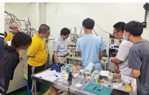
▲ Self-directed Learning Course: "Applications of Low-resistivity Metal Silicides and Semiconductors." Students learned the critical role of metal silicides in advanced semiconductor manufacturing processes. Photo: Instructor demonstrating the operation of a high-vacuum triple-target sputtering system.
