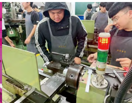
Micro-credit Course: "Manufacturing Techniques and Practical Applications of a Twin-cylinder Pneumatic Engine." Through intensive, hands-on training modules, students explored the relationship between machining parameters and manufacturing outcomes. Photo: Flywheel machining using a lathe.
